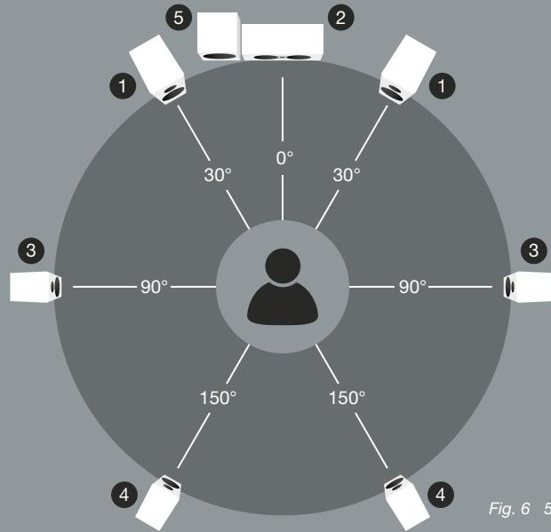
Fig. 6 5.1 and 7.1 multi-channel speaker setup.
