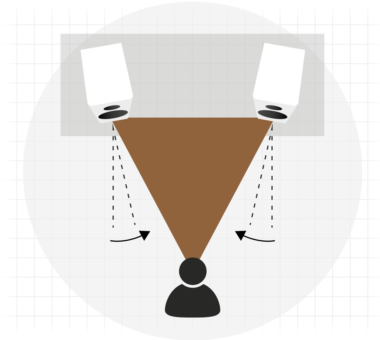
Fig. 5 Angle inwards loudspeakers to improve imaging.
